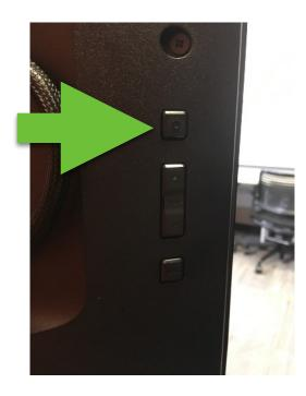
IMAGE: TOP button on the back of the right side of the TV(looking at rear side of TV) is the Power button to turn the TV on and off.
